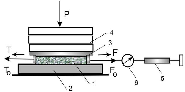
**Fig. 5.** Functional scheme of the test rig for study of starting friction.
